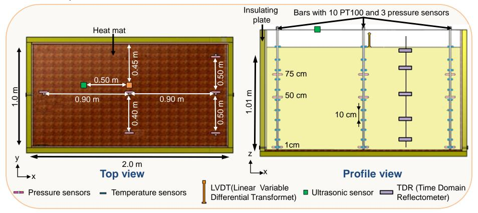
Measures: • Pressure fields, • Temperature profile, • Soil motion
