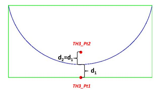
Fig. 1: TH3 case upper half geometry providing point locations of the new performance measures
