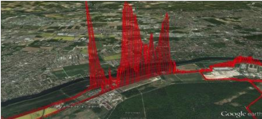
Above: Methane emissions in the surroundings of a Waste Water Treatment Plant near Conflans- Saint-Honorine (17. December 2012)
